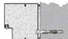
T90 BlockFrame with trimming profile Screw mounting with butt wall connection in fair-faced concrete/fair-faced masonry
