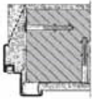
Corner frame Dowel mounting in plaster-coated wall surfaces
