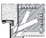
Corner frame T30 type H8-5 corner frame with combined masonry dowels
